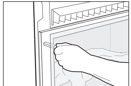
Figure (3) Remove front safety glass by firstly removing four dome nuts.
