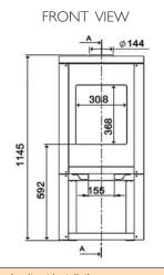
Dimensions shown above are in millimetres. Reference dimensions only. We recommend measuring individual units at installation.
